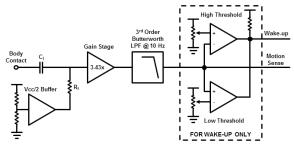
Figure 3. Block diagram of hardware for motion sensing. powered by two CR2032 3V lithium batteries: one for the eZ430-RF2500 transceiver and one for all other circuitry.
