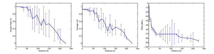
Fig. 5. Packet yield (*left*), link quality indicator (LQI, *center*), and received signal strength (RSSI, *right*) outdoors with the Telos mote and internal antenna. The results are averaged over 10 receivers co-located. From 75-110 feet, a dip in the terrain yields more erratic readings and wider variation in RSSI.
